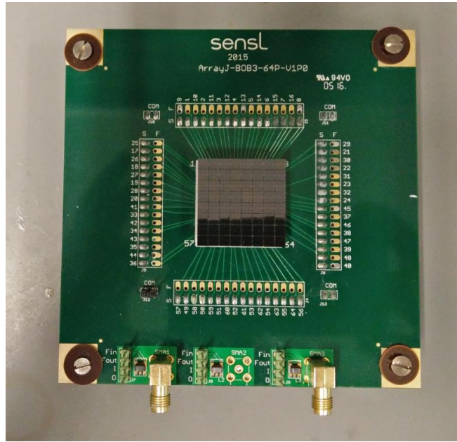
Figure 4.6 SiPM array SensL J-30035-64P-PCB with its breakout board.
